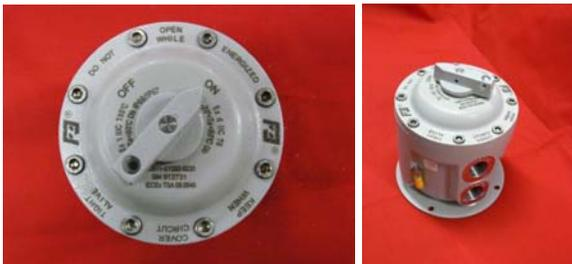
RJB11S1500 Explosion-proof isolator and selector switches up to 4p 32A 11kW AC3. Feature padlockable handle, cable entries in the bottom side or top-bottom. Mounting base with 4 fixing points. External equipotential bonding connection facility for 4-6 mm<sup>2</sup> wire.
